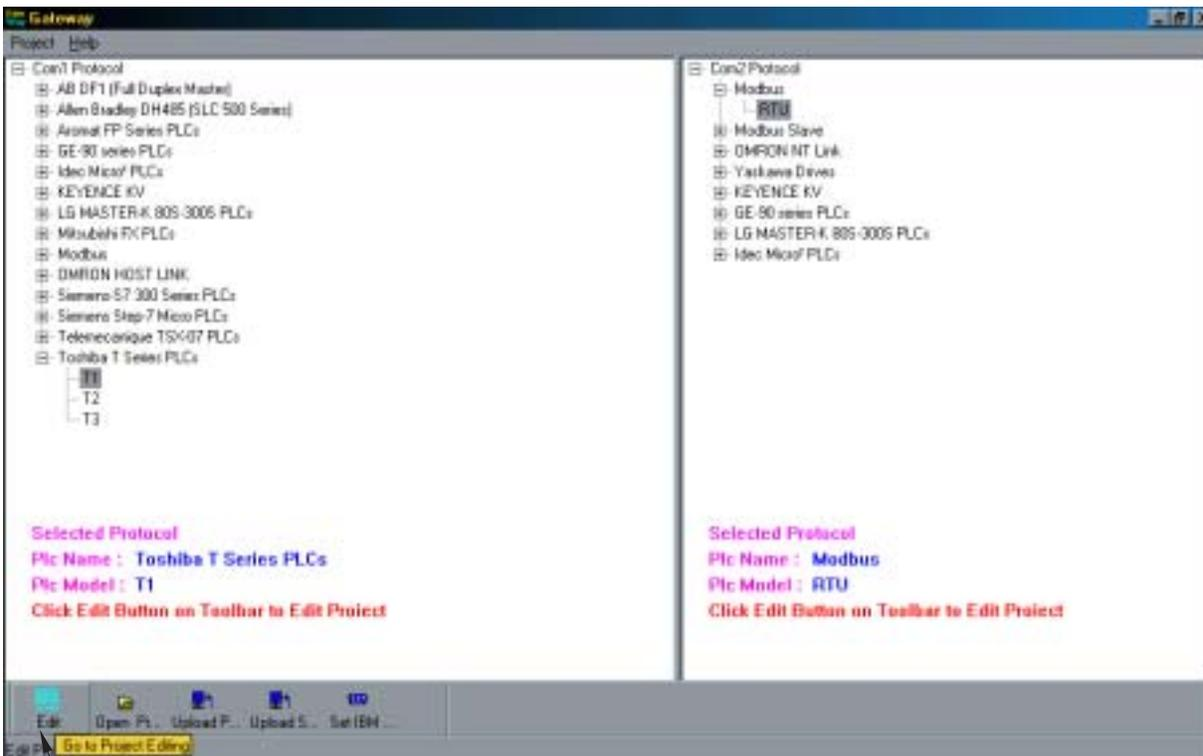
After the PLCs have been selected for both Com ports, click on the Edit Button. The Block edit screen should appear.
