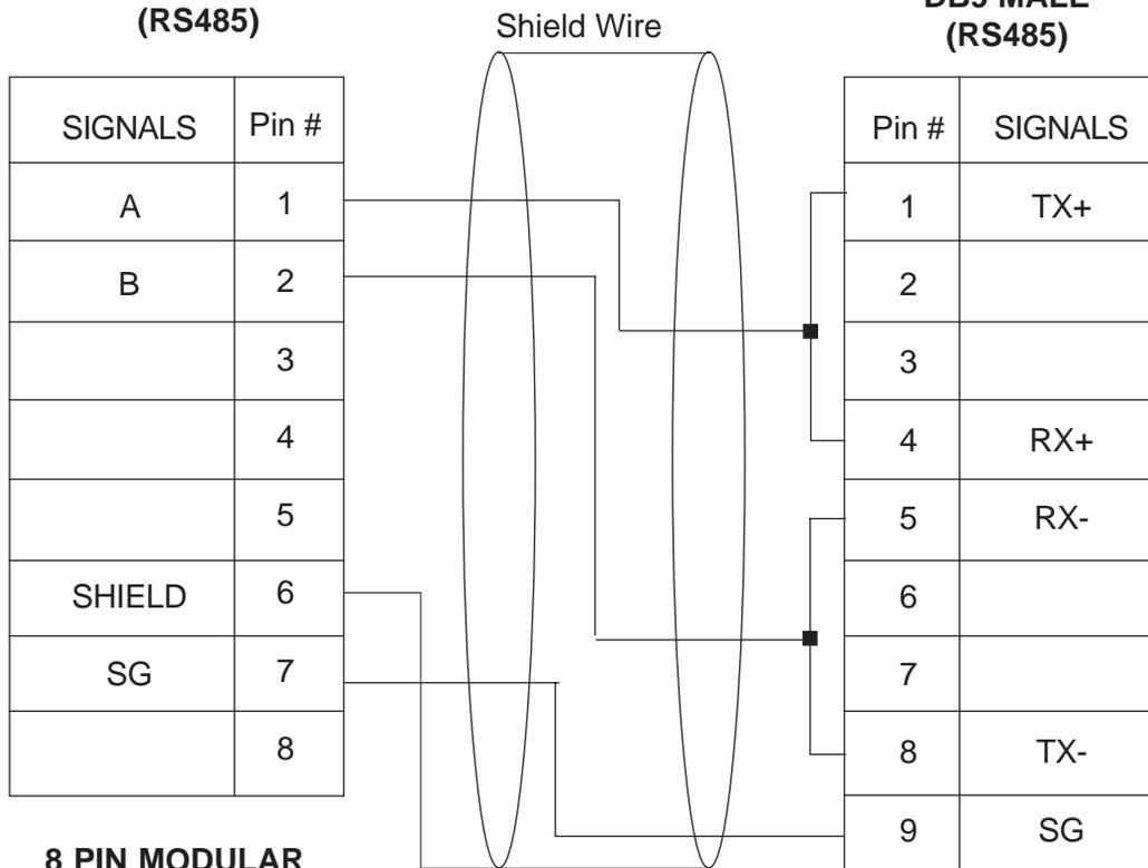
**8 PIN MODULAR CONNECTOR PINOUTS FRONT VIEW**
