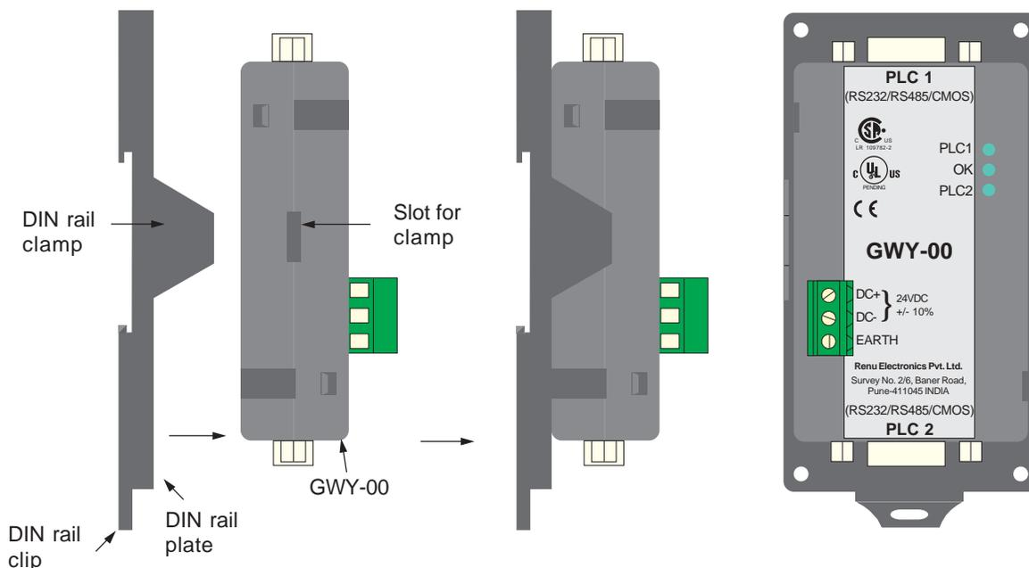
Following drawing shows the dimensional details of Gateway with DIN rail plate
