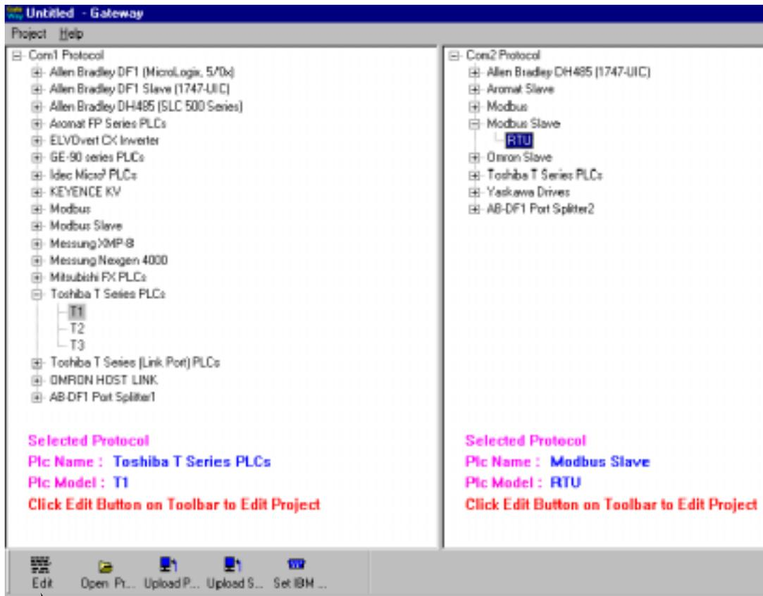
After the PLCs have been selected for both Com ports, click on the Edit Button. The Block edit screen should appear.
