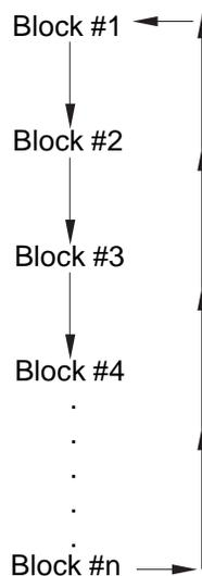
When Control word is enabled, it decides which block has to be executed by writing a specific data in the control word. Please refer to Example 4.1 for description on defining Blocks in Master - Master configuration.
