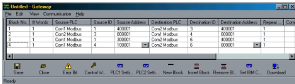
*Source PLC / Destination PLC: Setup Software appends 'Com1' and 'Com2' when protocols are same on both the ports.*
