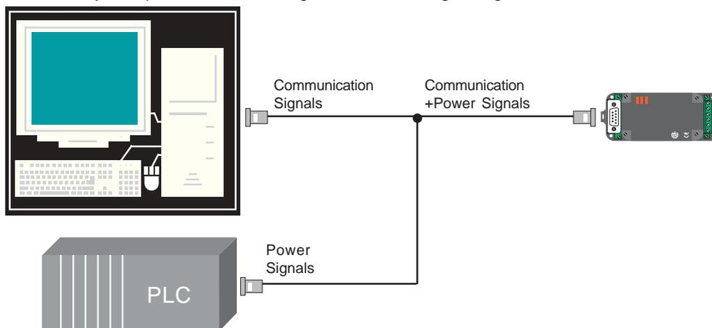
**GWY-04 and GWY-08** have RS485 PLC1 port hence RS232 to RS485 converter cable is required for Gateway Configuration. User can initiate IBM communication by leaving PLC ATTACH pin open. There is NO TIME-OUT for these models. Use Gateway Setup V1.xxx for creating and downloading configuration.
