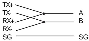
***Note: If user has attached shield to Earth on Device end, leave the shield open on Gateway end. If user has connected shield to Signal Ground on Device end, connect shield to Signal Ground on Gateway end.***
