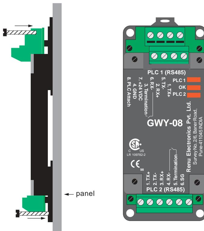
1. Insert screws in the holes provided on the DIN rail plate.
