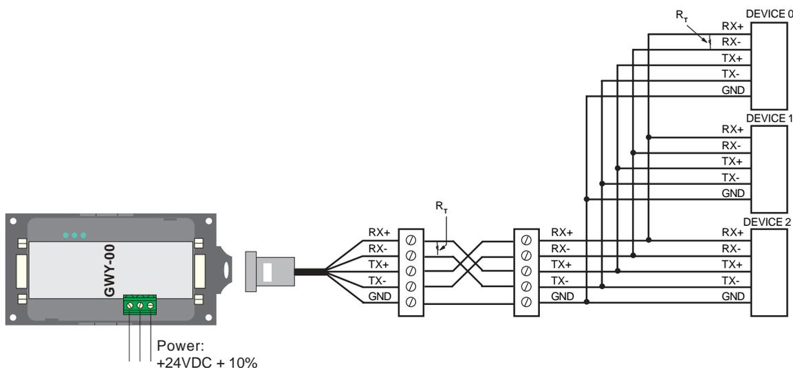
Note: User should add Termination resistor ( $R_T=180\text{ Ohm}$ ) in Receive lines of first and last node.
