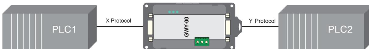
Connect each PLC to Gateway via the PLC's communications port (correct cables are required) and the PLCs can easily exchange information.
