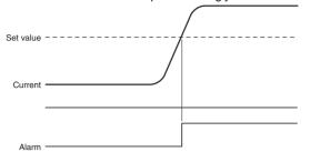
Transistor output models: ALM indicator lit, ALM transistor output Relay output models: ALM indicator lit, OR of all detection status output
