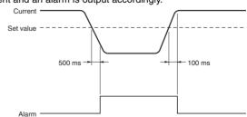
Transistor output models: ALM indicator lit, ALM transistor output Relay output models: ALM indicator lit, OR of all detection status output
