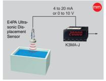
Monitoring liquid level in cleaning tanksWater tanks, devices using chemicals,
