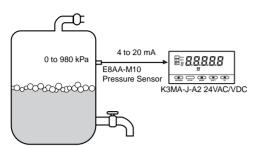
Here, the pressure inside the tank is to be displayed in units of 0.1 kPa.
