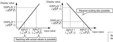
The decimal point can be optionally displayed. When displaying the decimal point, consider the number of digits to follow the decimal point prior to setting the scaling display value.
