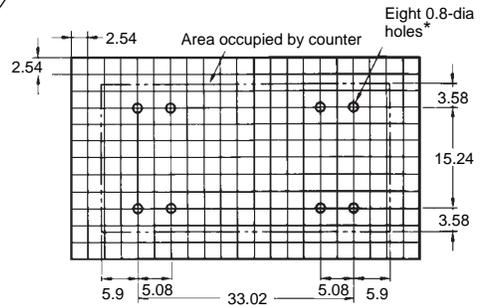
Note: Mounting hole dimensions conform to the pin pitch of a standard 28-pin IC socket.
