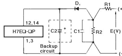
When the capacitor is used, its backup time can be calculated by the following formula\*:
