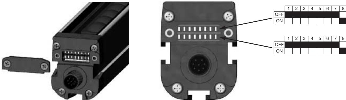
**There are two lines of dip switches in each transmitter and receiver. The settings must be done for both lines.** Change the setting of the dip-switch and close the cap again. The light curtain can now be reconnected to the power supply.
