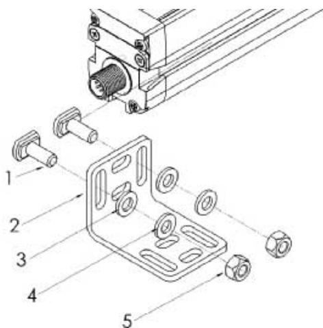
Note: Shipment contains different quantity of brackets, depending on the length of the LC. Longer LC contains a higher number of brackets, following the rule of every 400 mm one bracket.
