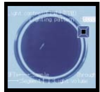
Detection of surface defects for button-type battery
