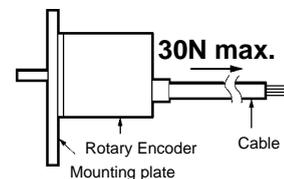
Do not pull the cable. Make sure that the E6A2 including its shaft is free of any shock.
