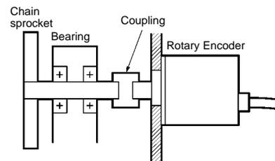
When inserting the shaft into a Coupling, do not strike the shaft or the Coupling with a hammer or subject any other shock to the shaft or Coupling.
