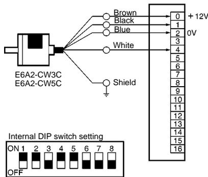
**Connection to C200H-CT□□ High-speed Counter Unit**
