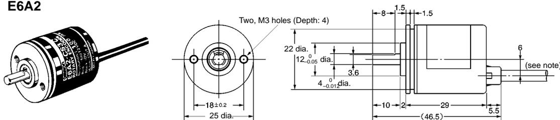
**Note:** Vinyl-insulated round cable with five cores, 4 dia. (0.16 dia. x 7), standard length: 500 mm
