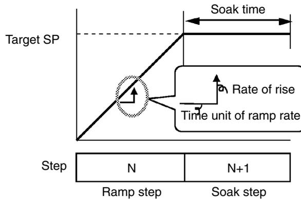
Set each of the above program elements in the “target SP 0 to 7”, “rate of rise 0 to 7” and “soak time 0 to 7” parameters.
