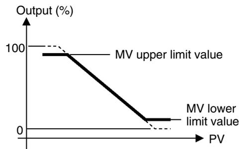
In heating and cooling control, the manipulated variable at the cooling side is treated as a negative value for the sake of convenience. The upper limit is set for the heating side (positive value), and the lower limit is set for the cooling side (negative value) as shown in the following figure.
