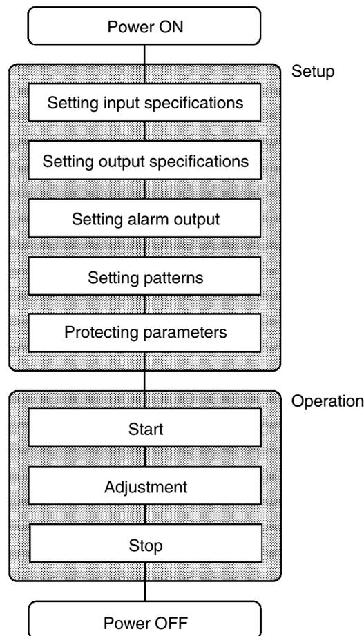
The descriptions in this chapter follow the order of basic operations shown in the flow above. Examples of operation of each of the items are described up to completion of parameter setup. However, you must move to the top parameter of the following Setting. For example, when you have finished “setting input specifications” and you want to “set output specifications,” move to the top parameter of “setting output specifications” from the bottom parameter of “setting input specifications.”
