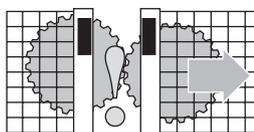
14. Do not mount the switch and actuator on magnetic materials, otherwise it may affect the operating distance.
