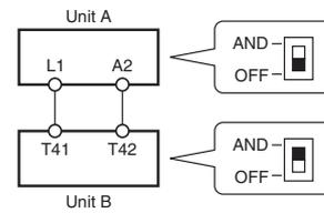
**Note:** A setting error will occur and Unit B will lock out if the logical AND setting switch on the Unit is set to OFF.
