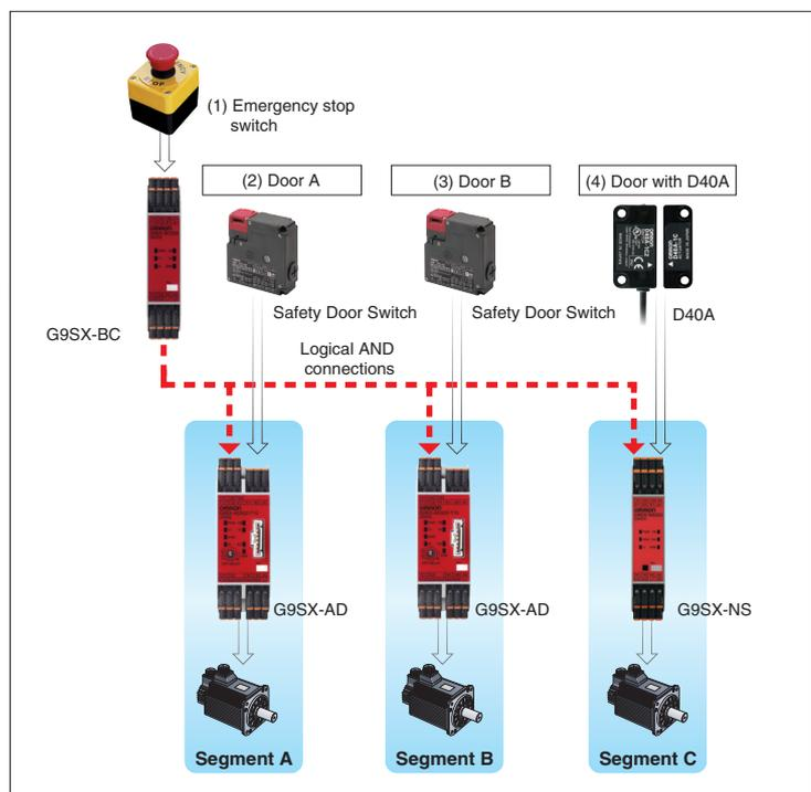
Note: Refer to the G9SX datasheet (Cat. No. J150) and to the 2006 Safety Components Series Group Catalog (Cat. No. Y106) for details on logical AND connections and the G9SX-series Controllers.
