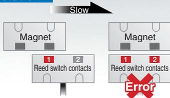
If the switching timing of reed switch contacts 1 and 2 varies too much, the Controller detects an error and turns OFF the output to maintain safety.
