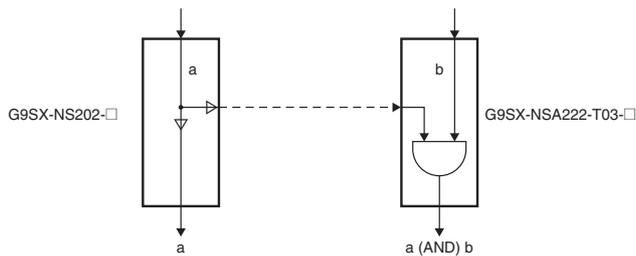
This is illustrated using the application in the following diagram as an example. The equipment here has two hazards identified as Robot 1 and Robot 2, and it is equipped with Non-contact Door Switches and an emergency stop button as safety measures. If the door to Robot 2 is opened, only Robot 2 is stopped (i.e., a partial stop). If the door to Robot 1 is opened or the emergency stop button is pressed, both Robot 1 and Robot 2 stop (i.e., a complete stop).
