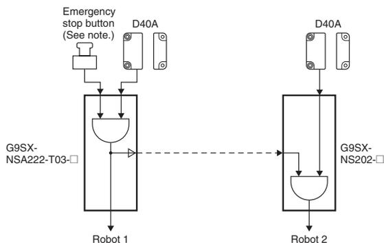
**Note:** A manual reset is required when an emergency stop is used.
