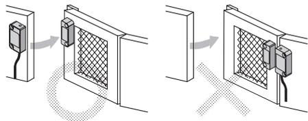
12. Where two or more Switches are mounted side-by-side, they must be no closer than 25 mm.
