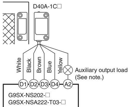
**Note:** The auxiliary output load current must be 10 mA max.
