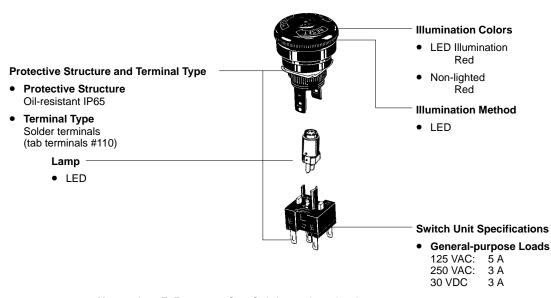
Note: A165E Emergency Stop Switch must be ordered as a set. No LED is installed for the non-lighted model.
