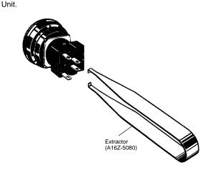
Grip the part between the Switch holder of the case and the Switch Unit using the A16Z-5090 Extractor, and pull to remove the Switch
